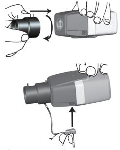
Figure 5.1 Mounting a lens
